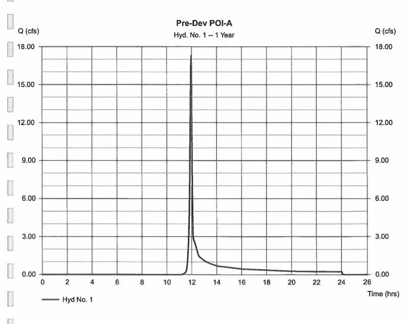
Hydraflow Hydrographs by Intelisolve v9.22
