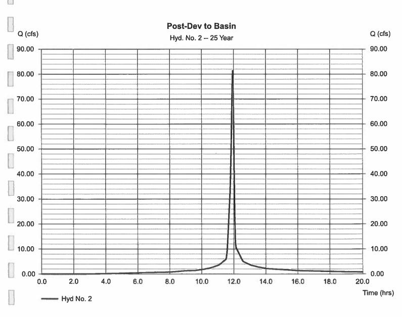
Hydraflow Hydrographs by Intelisolve v9.22
